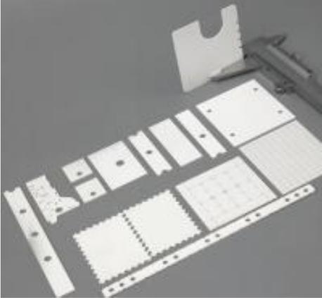
Alumina, also known as Aluminum Oxide, is a hard wearing advanced technical ceramic material frequently used in a wide variety of industrial applications. Once fired and sintered, it can only be machined using diamond-grinding methods. It features high hardness and wear resistance, low erosion levels, high temperature resistance, corrosion resistance, and bioinertness. Additionally, it can be highly polished making it useful for precision sealing applications like pumps and pistons.
