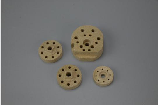
Cordierite ceramics are well known for their low thermal expansion and refractory character. Although cordierite is available as a powder, when we use the term we are generally talking about ceramic that went into the kiln as ordinary composite of ceramic powders but emerges as a cordierite crystalline matrix (grown by the firing process tuned to its needs).
