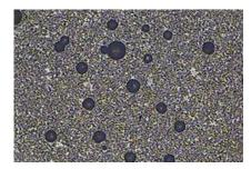
The crystal orientation of the Sintered Silicon Carbide +Spherical-pore material, and the spherical micropores are evenly distributed under the 200X optical microscope, and the micropore size is 50 to 80 µm.
