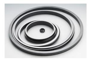
The Sintered Silicon Carbide+Spherical-pore is formed into micropores by adding a special pore-forming agent through high-temperature sintering, and the micropores uniformly distributed on the friction surface and independently connected, act as a reservoir of fluid or lubricant, and help promote The friction interface maintains the liquid film, reduces the frictional heat of the
