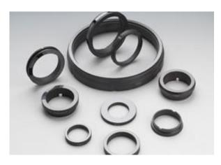
The Sintered Silicon Carbide+Graphite material is formed by sintering an atomic crystal composed of a strong covalent bond of Si-C and a flexible carbon in a vacuum sintering furnace at 2100 °C. The Sintered Silicon Carbide+Graphite have the properties of the original sintered silicon carbide material, such as strong corrosion resistance, wear resistance, high electrical conductivity and high temperature stability, and the
