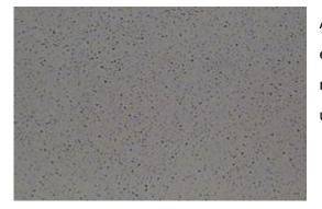
Sintered silicon carbide is sintered by pressureless sintering of submicron silicon carbide powder in a 2100 ° C vacuum sintering furnace. Due to its high-strength single-phase fine-grained structure at high temperatures, SSiC's high purity and high density make it highly resistant to corrosion, and its excellent surface finish makes it ideal for applications in mechanical seals and valves. , bearings and oil, chemical, aerospace, automotive and other fields.
