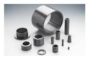
The reaction-sintered silicon carbide is formed by reacting and sintering submicron silicon carbide powder into free silicon (content less than 12%) and reacting it with free silicon in a vacuum sintering furnace at 1500 °C. The material has the characteristics of lubricity, small friction coefficient, wear resistance and strong plasticity, and the maximum outer diameter of the sealing ring can reach
