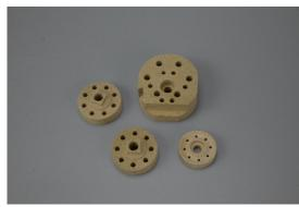
Cordierite ceramics are well known for their low thermal expansion and refractory character. Although cordierite is available as a powder, when we use the term we are generally talking about ceramic that went into the kiln as ordinary composite of ceramic powders but emerges as a cordierite crystalline matrix (grown by the firing process tuned to its needs).
