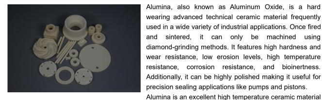
Alumina, also known as Aluminum Oxide, is a hard wearing advanced technical ceramic material frequently used in a wide variety of industrial applications. Once fired and sintered, it can only be machined using diamond-grinding methods. It features high hardness and wear resistance, low erosion levels, high temperature resistance, corrosion resistance, and bioinertness. Additionally, it can be highly polished making it useful for precision sealing applications like pumps and pistons.
