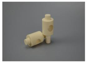
Alumina, also known as Aluminum Oxide, is a hard wearing advanced technical ceramic material frequently used in a wide variety of industrial applications. Once fired and sintered, it can only be machined using diamond-grinding methods. It features high hardness and wear resistance, low erosion levels, high temperature resistance, corrosion resistance, and bioinertness. Additionally, it can be highly polished making it useful for precision sealing applications like pumps and pistons.
